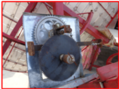
Close up of sun tracker. Made mostly of bike parts!
